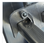
Extending section locking hooks
